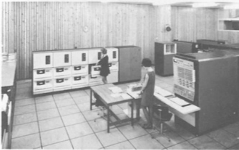
The central processor multiple disc and drum storage units of the IBM 360/67 computer.
